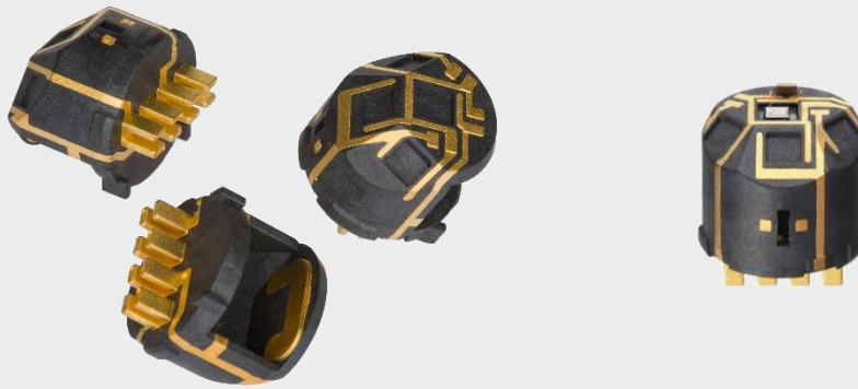
Figure 1: Sun sensor in MID design supports climate control in cars
