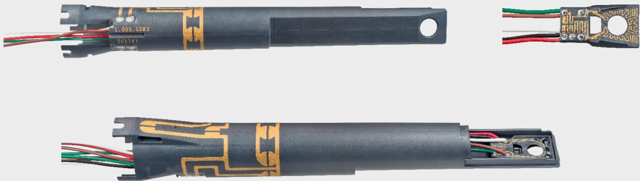
Figure 1: Optics carrier (top left) and heating element (top right), shown separately and assembled (bottom)
